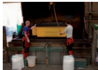
The powder transforms to liquid creating a plastic skin inside the mould.
