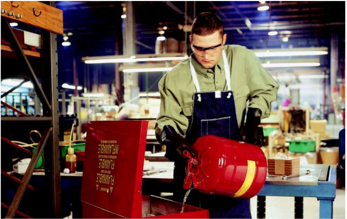
RISKY: Only the minimum quantity of a flammable substance should be present in the actual work area.
